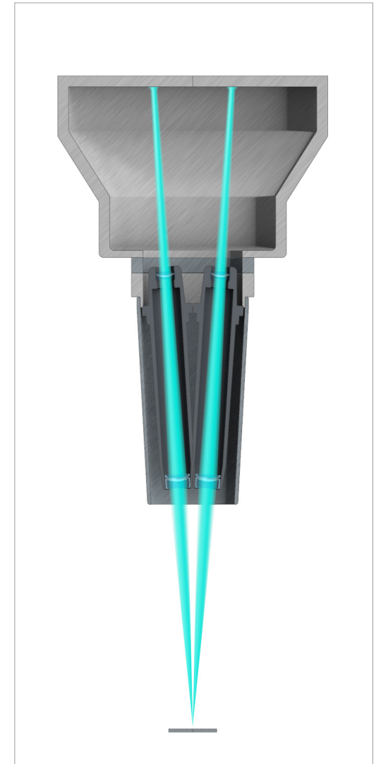
Schematic beam path of a Greenough type stereo microscope.
